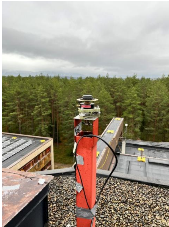
Figure 7-1: Pillar with the u-blox antenna used for the four u-blox F9P receivers.
