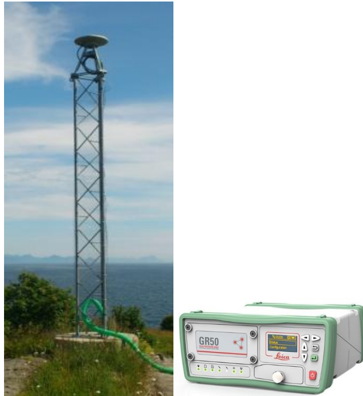
Figure 3-1: Example of antenna and receiver for a permanent reference station. Credits: NMA, Leica Geosystems.
