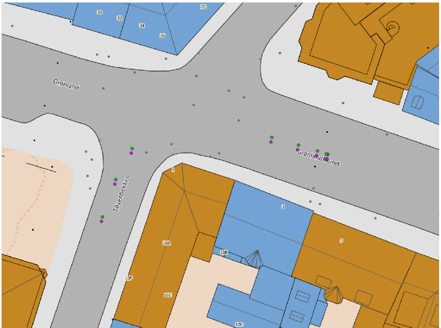
Figure 6-5: Example 3, large position errors, possibly incorrect ambiguity resolution. HyPos-SSRZ, full configuration, with Teria PYX. Only fixed solutions are shown.
