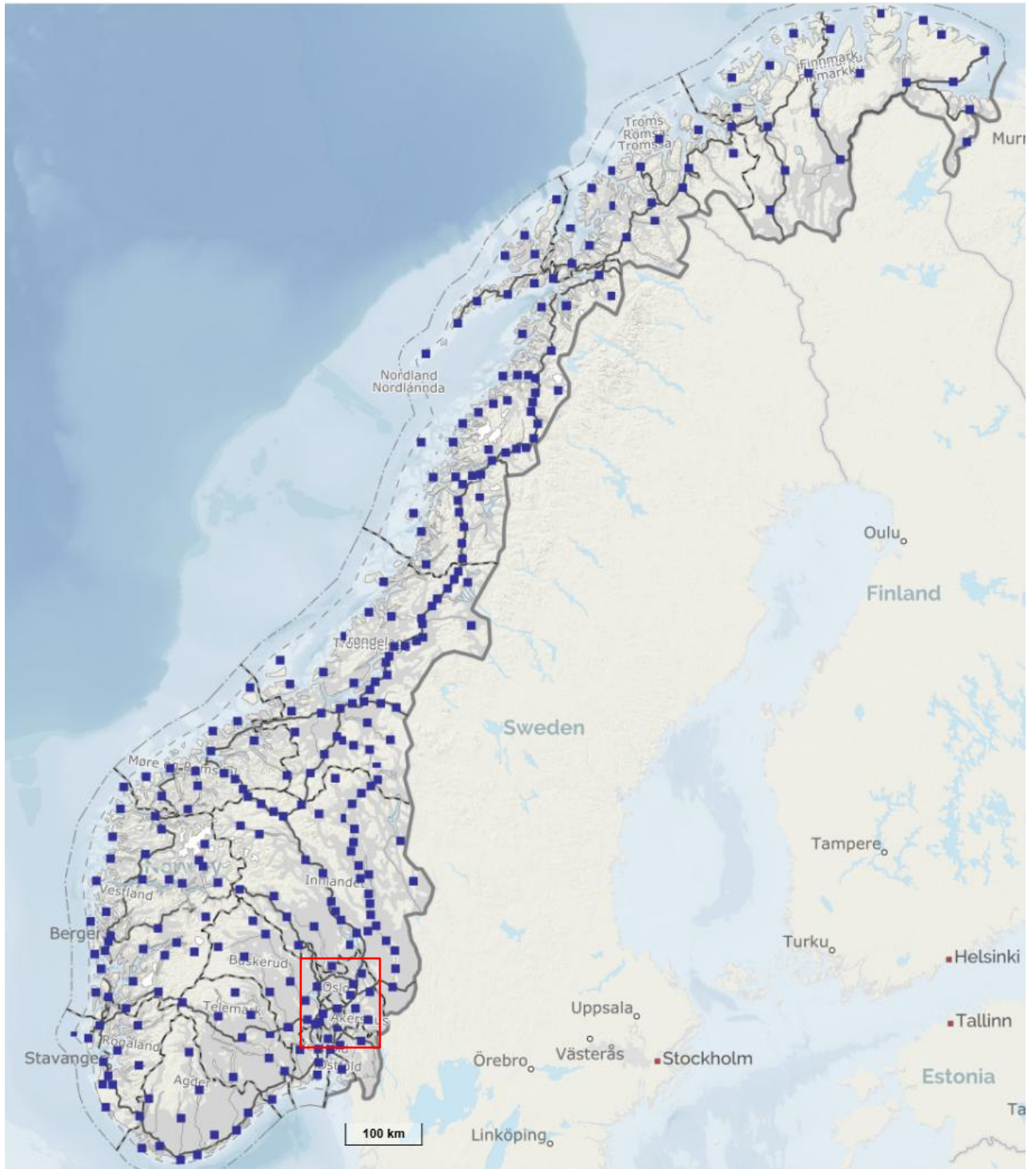
Figure 3-2: NMA's permanent reference stations. HyPos_SSR subset is inside the red rectangle.
