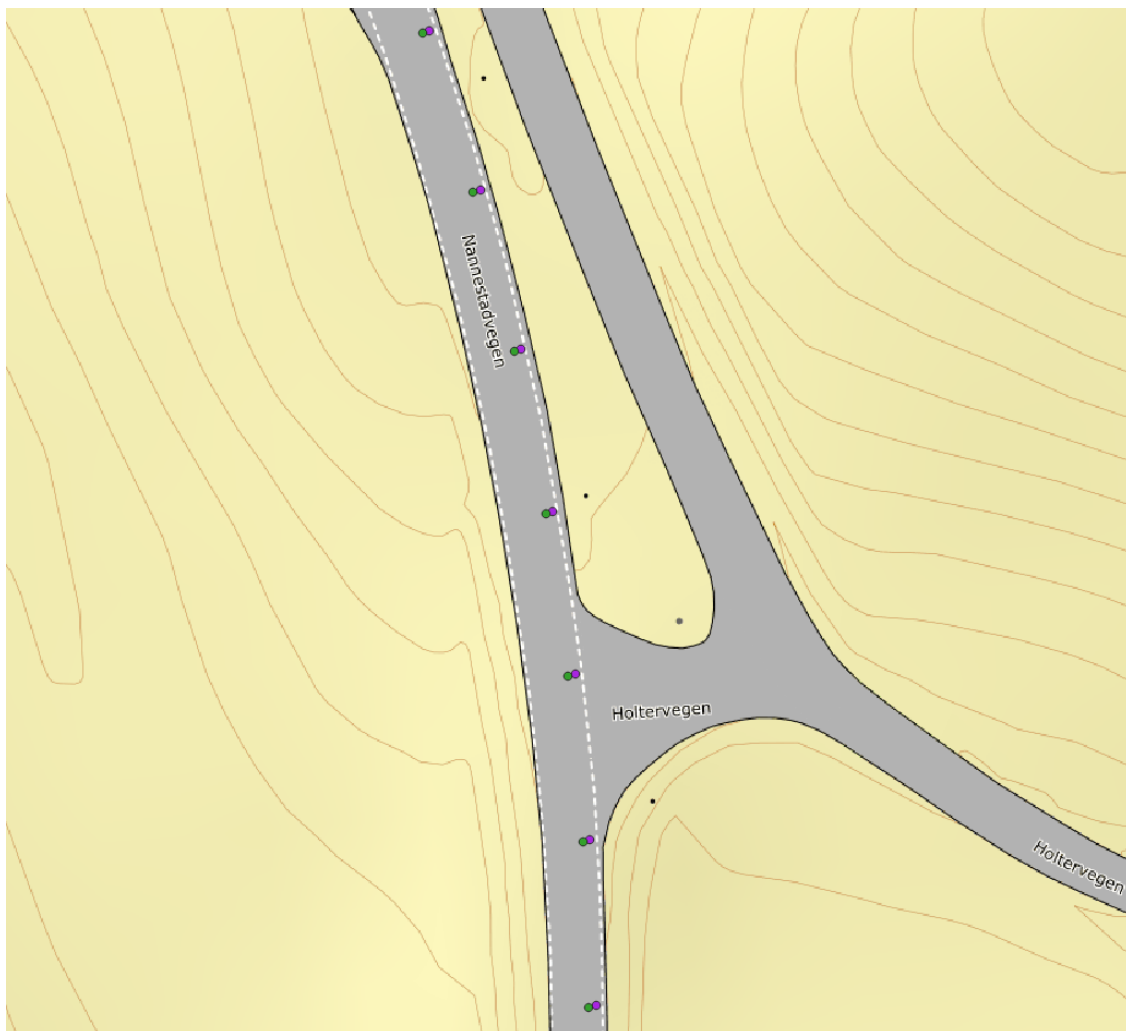
Figure 6-4: Example 2, large position errors, possibly incorrect ambiguity resolution. HyPos-SPARTN, full configuration, with u-blox F9P.
