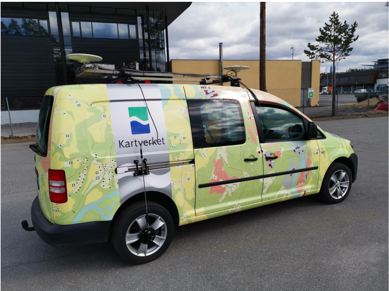
Figure 4-1: Measurement vehicle. More antennas have been added since this photo was taken.
